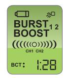
((((((O)))))) Power Bar: This shows the output from 0 to 15 for both left and right channels. Each segment represents approximately 7% of the total output.
